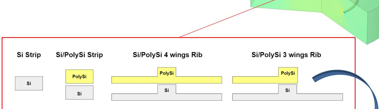
In the case of the rib waveguides, we have non uniform diffusion of free carrier, because the photo-generation rate generates electron-hole pair in the middle of the rib that diffuse along the lateral wings.
