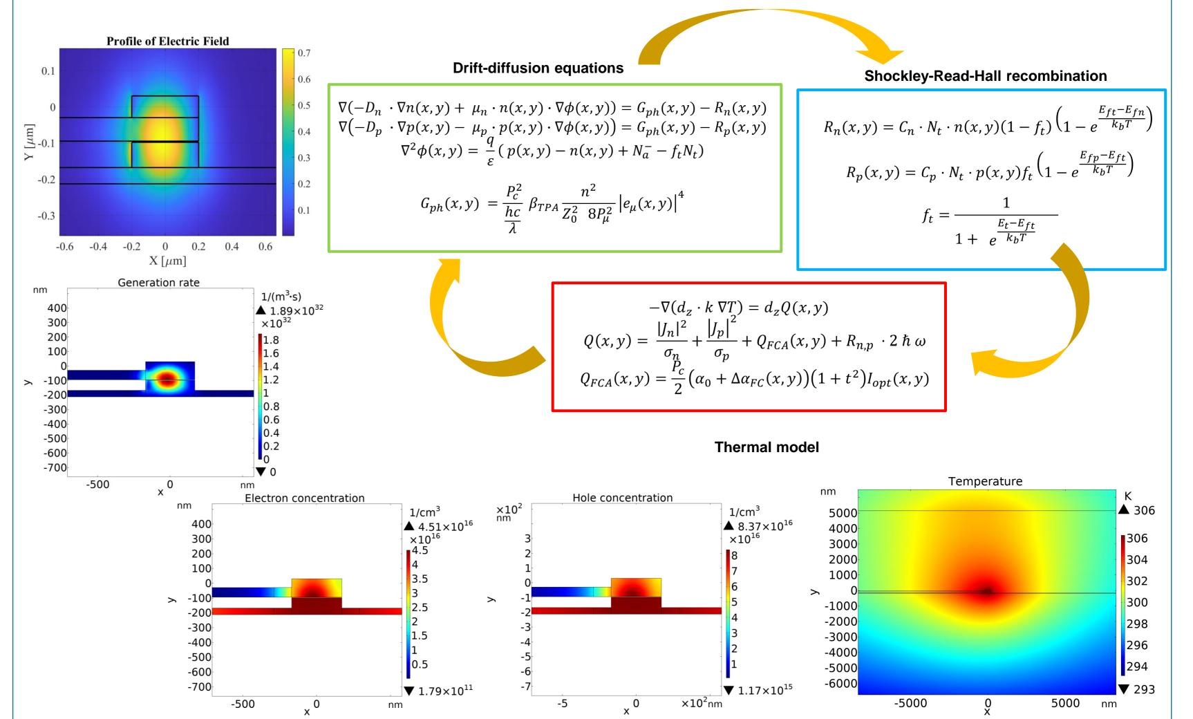
the circulating power  $(P_c)$  that refers to the energy of the light stored inside the ring. It depends on bus power and quality factor. We consider a silicon MRR, where there are two mainly type of non linear effect limiting the maximum power entering the waveguide: Two Photon Absorption (TPA) and Free Carrier Absorption (FCA).
