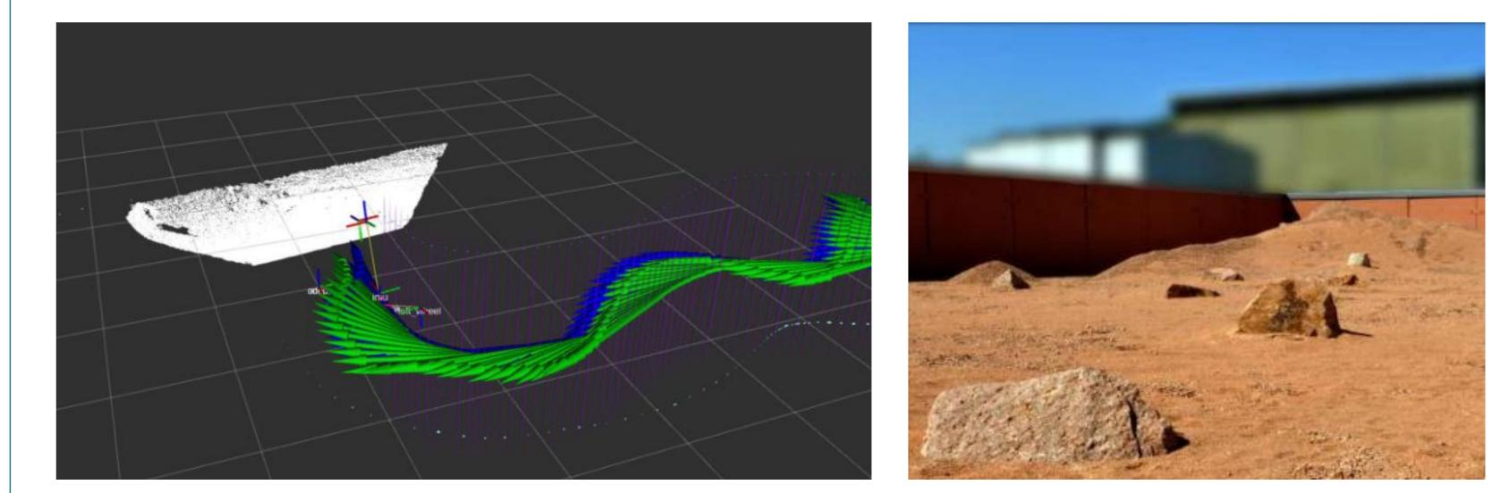
Global tracking and mapping: the pose graph optimized by the local tracking module will be wrapped in a higher-level global graph, which will include loop closure detections as well as tracked landmark locations. The global graph models the mapped environment and the corrected robot trajectory. Graph optimization will take place in a dedicated thread at a lower rate or triggered by a loop closure detection.
