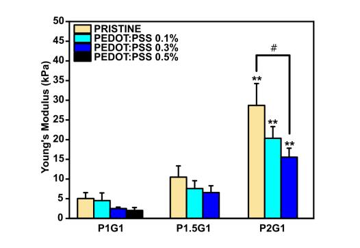
Elastic modulus of hydrogels increased by increasing PEGDA:gelatin ratio. Notably, the obtained values of stiffness matched the range of healthy cardiac tissue (≈10–30 kPa).
