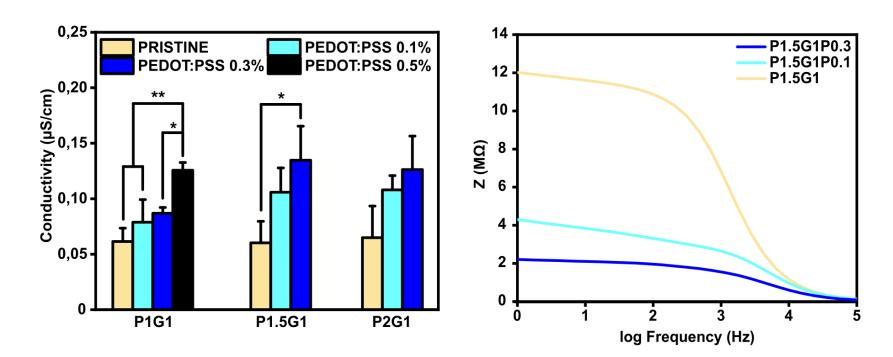
Surface conductivity increased as a function of PEDOT:PSS content. Moreover, hydrogels containing PEDOT:PSS possessed lower impedance (Z) than pristine hydrogels.
